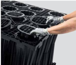
Polypropylene top covers are added to the top layer of the tank to fill the openings of the pillars and to ensure consistent support for the cover fill material.
