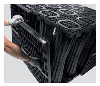
Polypropylene side panels are added to the perimeter of the tank to give lateral support against surrounding soils. The side panels have cutting guides which can be cut out using a jigsaw for the connection of plastic pipes.
